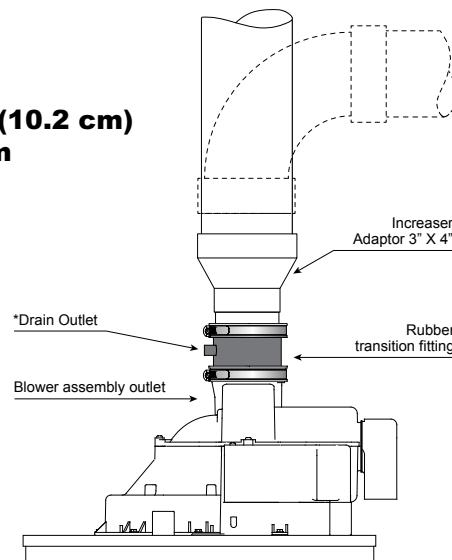
\* A plastic tube can be attached to the drain outlet to evacuate any condensate. For more information, consult the owner's manual, section Condensation in the venting system.
