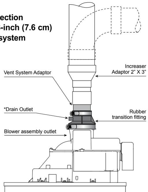
\* A plastic tube can be attached to the drain outlet to evacuate any condensate. For more information, consult the owner's manual, section Condensation in the venting system.
