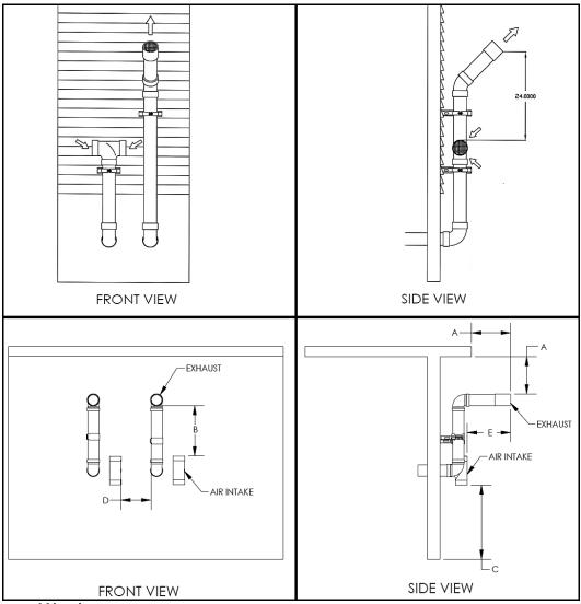
Figure 14: Horizontal Venting - NOTE: Drawing is meant to demonstrate system venting ONLY.
