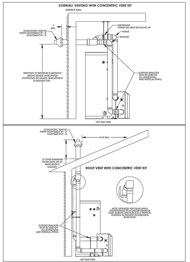
Figure 12: Concentric Venting - NOTE: This drawing is meant to demonstrate system venting only. The installer is responsible for all equipment and detailing required by local codes.
