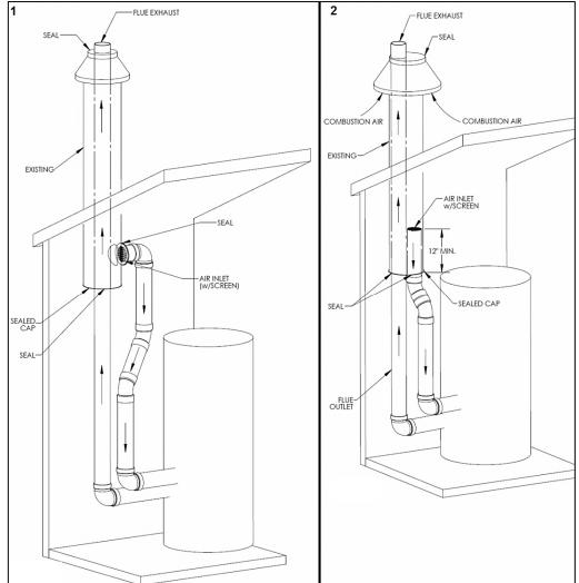
Figures 15-1 & 15-2: Concentric Venting - NOTE: Drawing is meant to demonstrate system venting ONLY.
