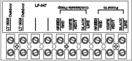
Figure 20: Low Voltage Wiring
