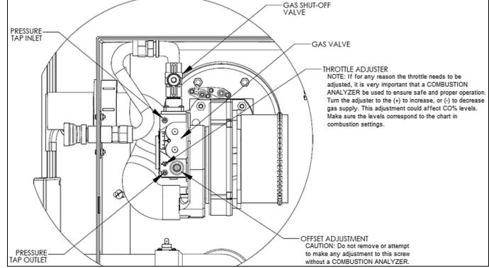
Figure 24: Gas Valve LP-179-P
