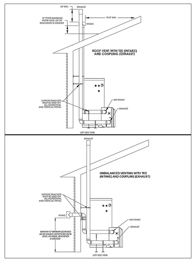
Figure 13: LP-179-F - NOTE: This drawing is meant to demonstrate system venting only. The installer is responsible for all equipment and detailing required by local codes.
