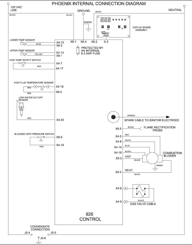
Figure 21: Wiring Diagram
