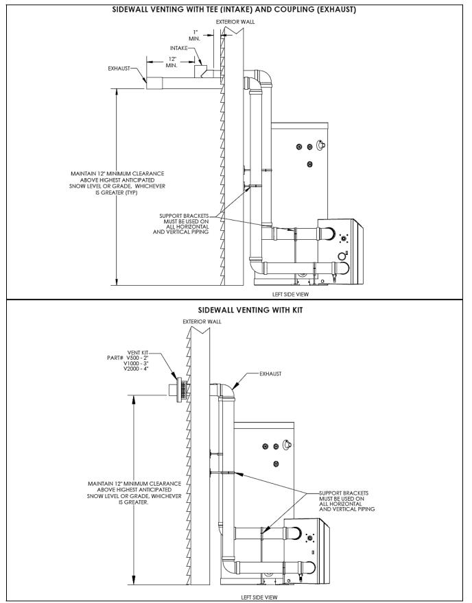
Figure 11: Sidewall Venting - NOTE: This drawing is meant to demonstrate system venting only. The installer is responsible for all equipment and detailing required by local codes.
