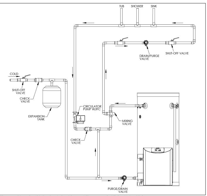
Figure 9: Phoenix with Recirculation Line and Thermostatic Mixing Valve Piping
