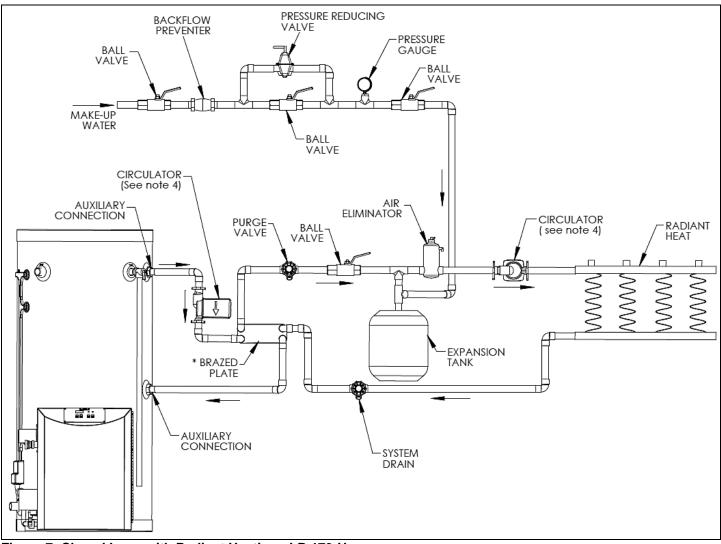
Figure 7: Closed Loop with Radiant Heating - LP-179-U
