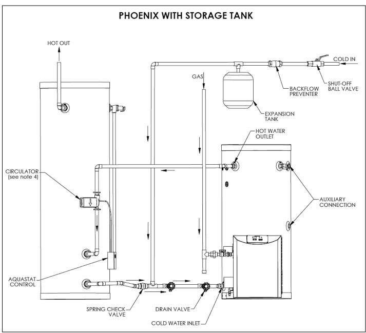
Figure 8: Phoenix With Storage Tank
