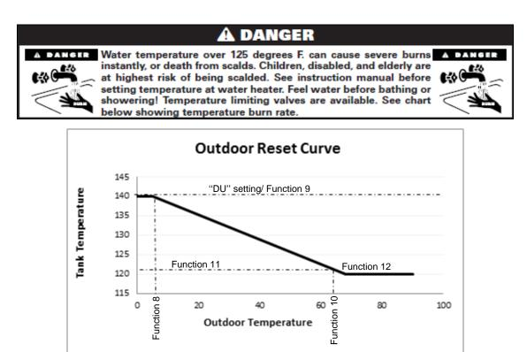
Figure 25 - NOTE: The maximum tank temperature is 160°F (71°C), independent of all settings described above.
