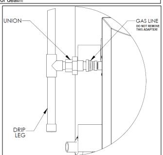
Figure 23: Phoenix Gas Connection - LP-179-Q
