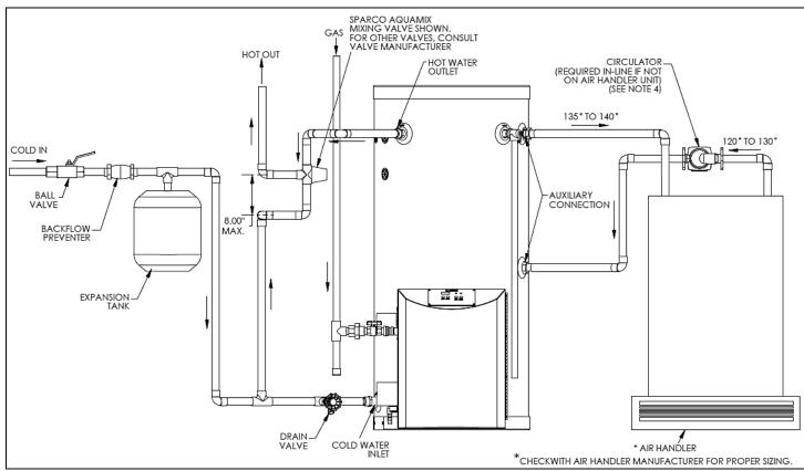
Figure 5: Phoenix with Air Handler on Side
