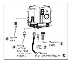
Figure 38 - Gas Control Valve Connections
