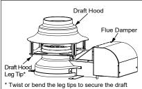
\* I wist or bend the leg tips to secure the draft hood to the flue damper.
