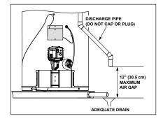
Figure 17 - Temperature and Pressure Relief Valve Pipe (Discharge Pipe)
