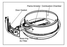
Figure 43 - Combustion Chamber
