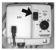
Figure 36 - Move switch to OFF position.
