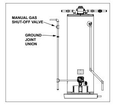
Figure 39 - Ground Joint Union Connection
