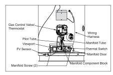
Figure 41 - Front view of water heater with outer door removed.
