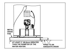
Figure 15 - Metal drain pan piped to drain.
