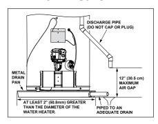
Figure 7 - A metal drain pan piped to an adequate drain can help protect flooring from leaks and drips.
