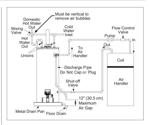
Figure 4 - Combustion Space Heating and Potable Water (Typical Installation)
