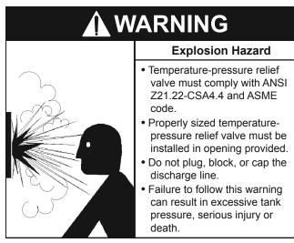
This water heater is provided with a properly rated/sized and certified combination Temperature-Pressure Relief Valve (T&P valve) by the manufacturer. The valve is certified by a nationally recognized testing laboratory that maintains periodic inspection of production of listed equipment of materials as meeting the requirements for **Relief Valves for Hot Water Supply Systems, ANSI Z21.22-CSA 4.4**.
