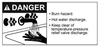
It is recommended that the temperature-pressure relief valve be checked to ensure it is in operating condition at least once a year.
