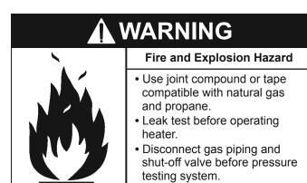
Use pipe joint compound or Teflon<sup>®</sup> tape marked as being resistant to the action of gases.
