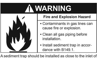
A sediment trap should be installed as close to the inlet of the water heater as practical at the time of water heater installation. The sediment trap should be either a tee fitting with a capped nipple in the bottom outlet or other device recognized as an effective sediment trap. If a tee fitting is used, it should be installed in conformance with the method of installation shown in Figure 15.
