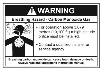
This heater is approved for operation up to 3,079m (10,100') without alteration.
