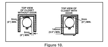
A WARNING Breathing Hazard - Carbon Monoxide Gas • Install water heater in accordance with the instruction manual and B149.1. • To avoid injury, combustion and ventilation air must be taken from outdoors. • Do not place chemical vapour emitting products near water heater. Breathing carbon monoxide can cause brain damage or death. Always read and understand instruction manual.
